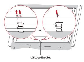
2 After removing the screw, remove the LG Logo Bracket. Attach the LG Logo Bracket with the screws, aligning it with the hole on the right side.
